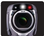
Visible Light Pictures Align with Thermal Images: 3.1MP Digital Camera, LED Lamp, and Laser Pointer
